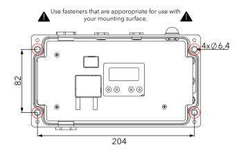
Drill holes to the surface according to holes spacing. Mount E-box via mounting holes on the surface.
