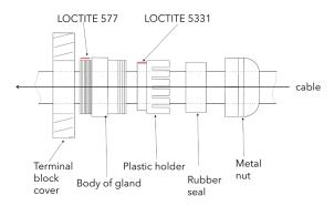
We recommend to apply an adequate layer of the paste LOCTITE 5331 on the plastic holder of the cable gland before inserting in into the body of the gland and an adequate layer of the paste LOCTITE 577 on the thread of the gland body.
