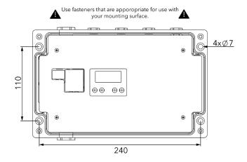
Drill holes to the surface according to holes spacing. Mount E-box via mounting holes on the surface.
