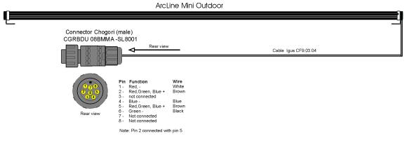
2. Adapter cable Chogori -RJ45 (it is not a standard part of delivery), for indoor use only
