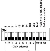
DIP 10 - if switched to ON=test light (the fixture lights at 3200K)
