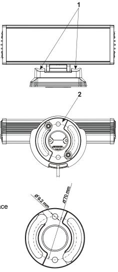
2. Turn the internal adjustable holder (2) to the position as shown on the picture and take it out from the base.
