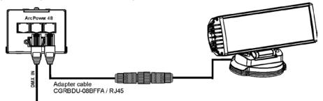
Connect the ArcPad 48 's cable to the ArcPower 48 via the adapter cable Chogori/RJ45. The power/data cable that connect the ArcPad 48 to the ArcPower48 has the following wiring:
