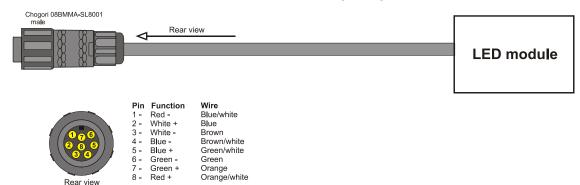
Adapter cable Chogori/ RJ45 betwen fixture and LED driver
