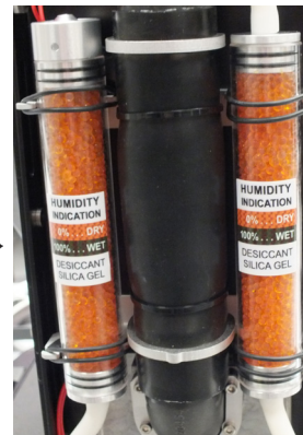
Silica gel desiccants in the fixture arm
